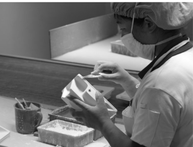
↑ Repairing the small bubbles
