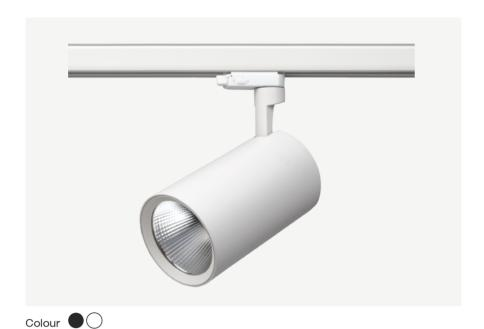
For use in retail, commercial, and residential accent lighting applications, designed for the illumination of merchandise or artwork. T55 is track mounted miniature LED spotlight fixture with integral driver. Offered in 3000K with a CRI of 90-plus, the fixtures are available in Max36W. Beam spread options include 15 degree, 24 degree, and 36 degree. Fixtures are available in white, black.
