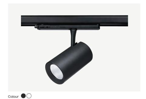
For use in retail, commercial, and residential accent lighting applications, designed for the illumination of merchandise or artwork. T56 is track mounted miniature LED spotlight fixture with integral driver. Offered in 3000K with a CRI of 90-plus, the fixtures are available in Max32W. Beam spread options include 18 degree, 24 degree, and 36 degree. Fixtures are available in white, black.
